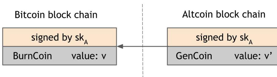
**Figure 10.2: Allocating altcoins via proof-of-burn.** The altcoin supports a GenCoin transaction that takes a *Bitcoin* transaction as input. GenCoin is signed by the same private key that signed the proof-of-burn (and using the same signature scheme). This ensures that the same user who burned bitcoins also created the GenCoin. If the peg ratio is 1:1, then  $v'$  must be no greater than  $v$ .
